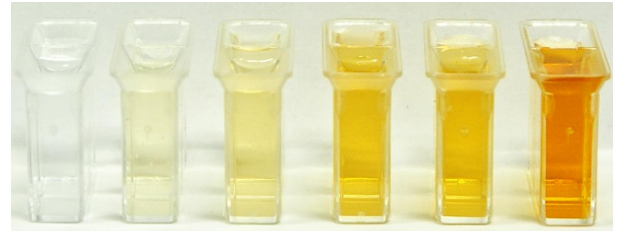
Fig. 4. Extracts of humic acid corresponding to 0, 4, 8, 20, 30, and 50 \text{ g kg}^{-1} of soil organic matter from left to right.
